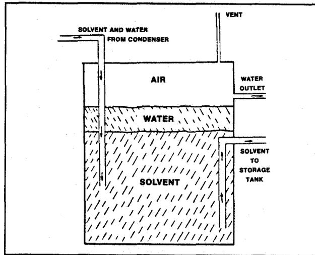
Figure 1. Diagram of a Water Separator
